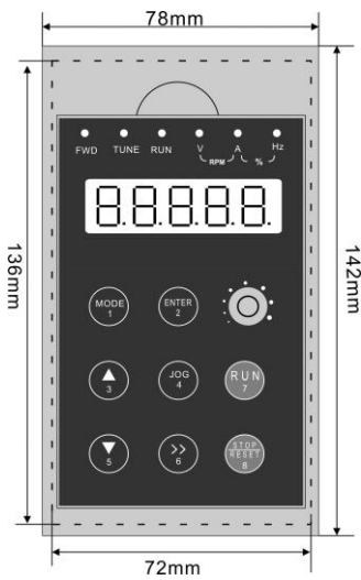
Installation dimension of Keyboard Booth: 136*72mm
