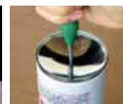
Piercing empty spray can for safe disposal
