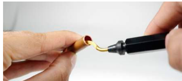
Remove Burr from inner
